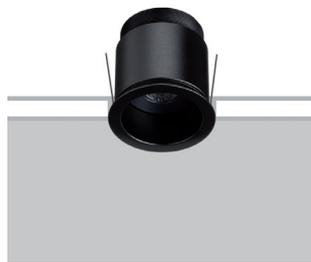
The Jimbo range of recessed fixtures offers adjustable optics in which, by working on an adjustment element, it is possible to change the opening of the light beam from 10° to 55°, in order to adapt to the project needs.
